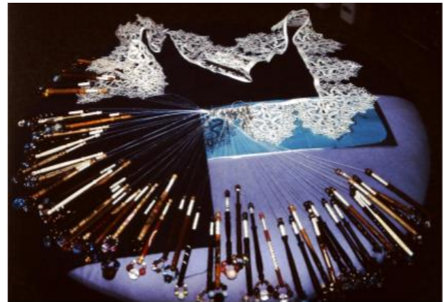
Fig. 6. The making or "growing" of the bobbin lace. The use of many bobbins for working on a single piece of bobbin lace reflects the complexity of the craft and the knowledge of the technique required to interlace the threads, follow the pattern and actualize the design.
